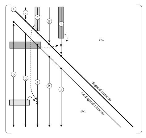
Figure 2.3.1. Crout's algorithm for *LU* decomposition of a matrix. Elements of the original matrix are modified in the order indicated by lower case letters: a, b, c, etc. Shaded boxes show the previously modified elements that are used in modifying two typical elements, each indicated by an "X".
