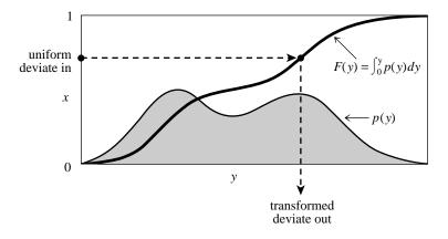
Figure 7.2.1. Transformation method for generating a random deviate y from a known probability distribution p(y). The indefinite integral of p(y) must be known and invertible. A uniform deviate x is chosen between 0 and 1. Its corresponding y on the definite-integral curve is the desired deviate.
