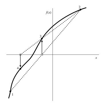
Figure 9.2.1. Secant method. Extrapolation or interpolation lines (dashed) are drawn through the two most recently evaluated points, whether or not they bracket the function. The points are numbered in the order that they are used.
