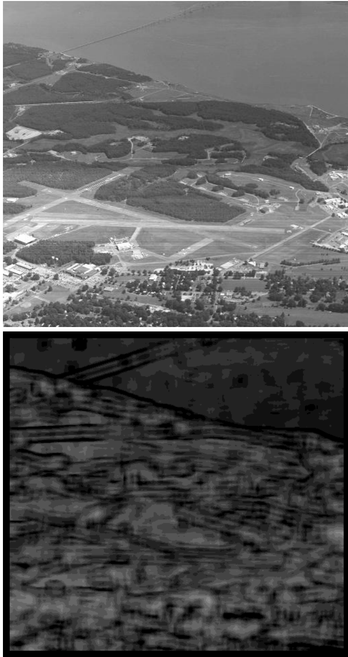
Figure 5.37: An aerial photograph (above) and an image representing the fractal dimension at each point in the scene (lower). Points of lower fractal dimension are darker. (Images courtesy Naval Surface Warfare Center, Dahlgren, Virginia.)
